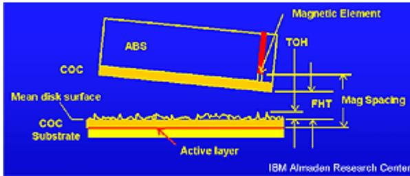
**Figure 3. Magnetic Spacing Component Roadmap**
