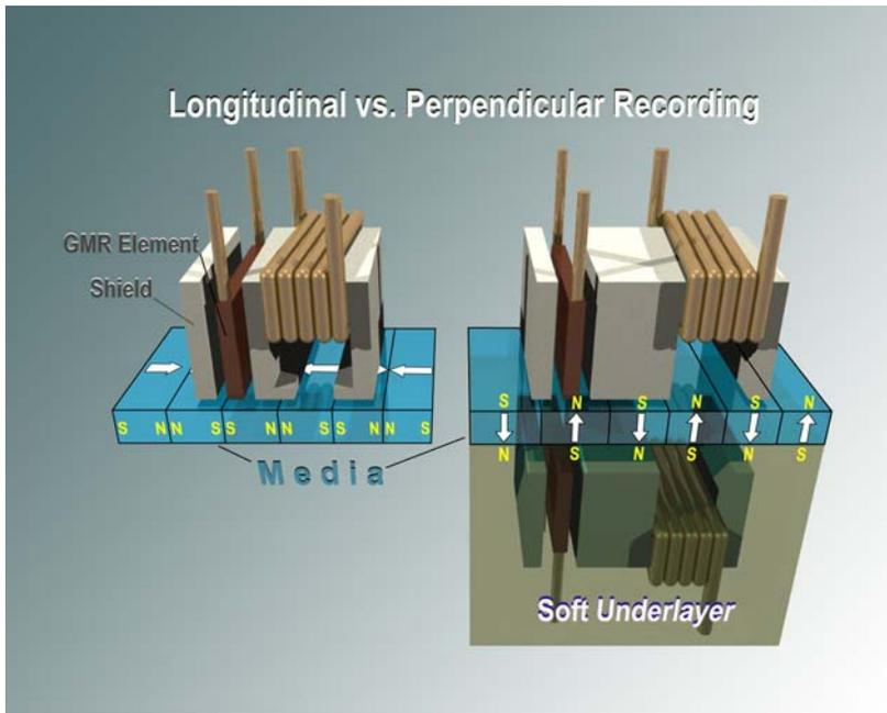
Perpendicular recording has its own special issues however. In order to maintain a consistent write field on the media the spacing between the head and the disk must have a lower flying height and tighter spacing loss tolerance and the write head poles require special shaping in order to prevent write fields going through the media soft magnetic layer to weaken and even overwrite adjacent track data.
